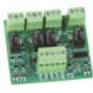
I/O expansion card - 4 OUTPUT 24VDC 1A - 4 INPUT
