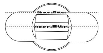
4. Hold the special tool and knob cover firmly at the same time and turn them together 1-2° clockwise first and then counter-clockwise.
